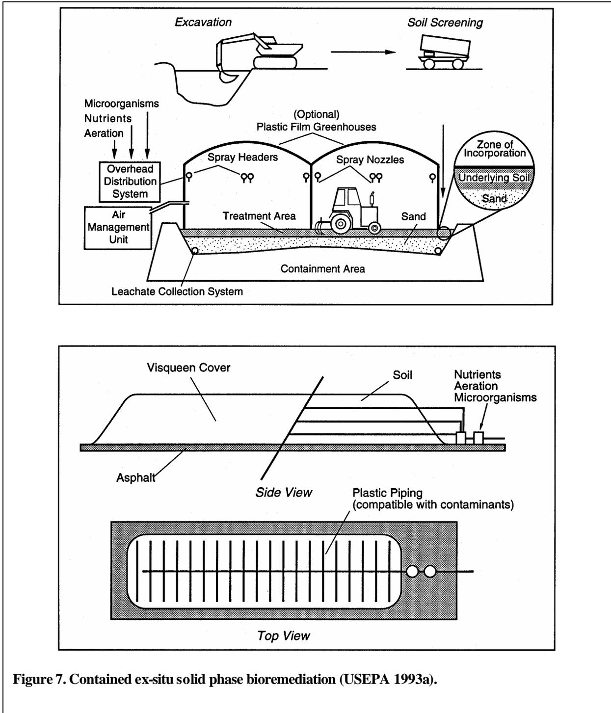
Figure 7. Contained ex-situ solid phase bioremediation (USEPA 1993a).
