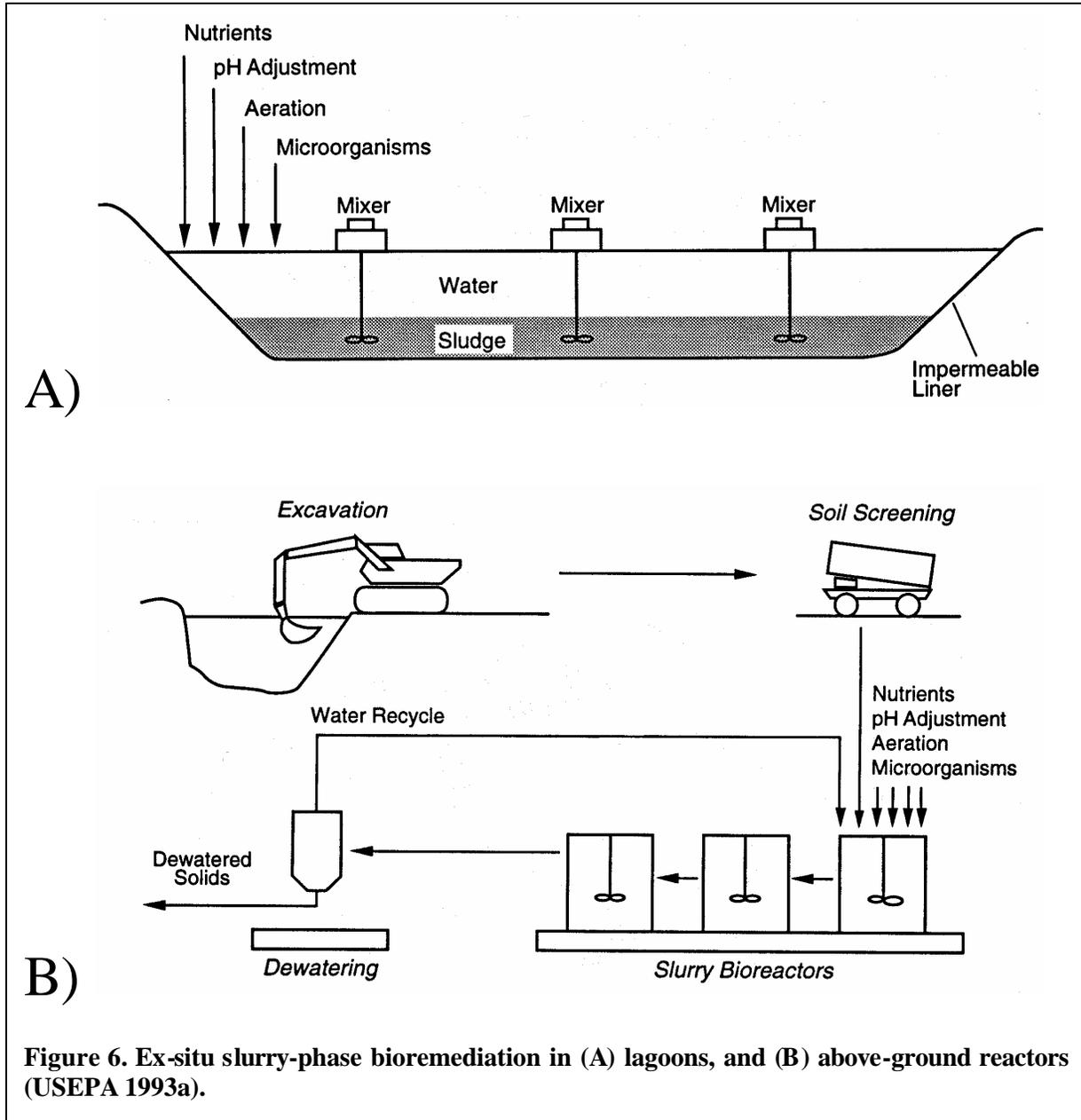
**Figure 6. Ex-situ slurry-phase bioremediation in (A) lagoons, and (B) above-ground reactors (USEPA 1993a).**
