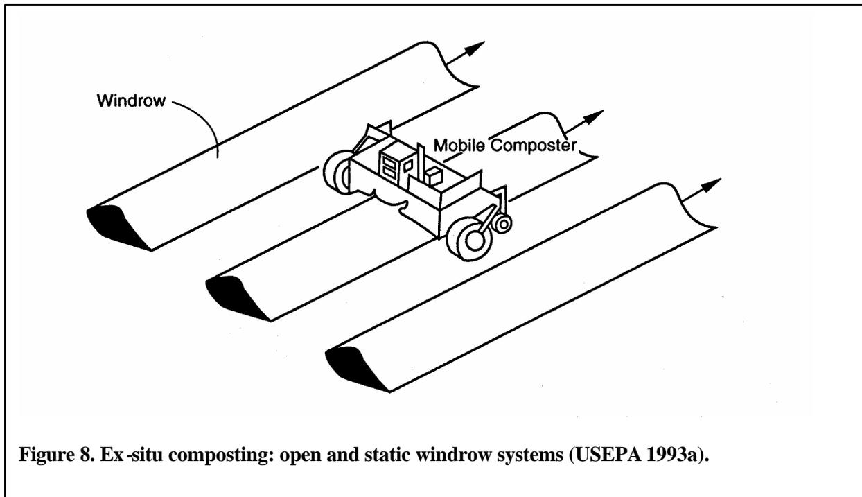
**Figure 8. Ex-situ composting: open and static windrow systems (USEPA 1993a).**
