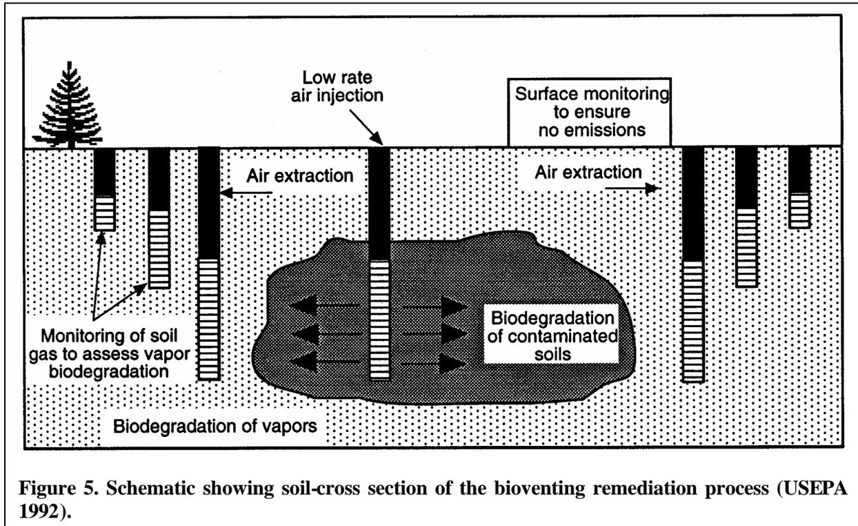
Figure 5. Schematic showing soil-cross section of the bioventing remediation process (USEPA 1992).
